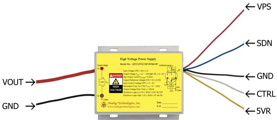
Figure 2. The Connecting Lead Wires of AHV24V15KVR5MAW
